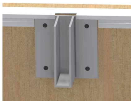
Figure 21 – Glass fin support bracket with upstand top trim
