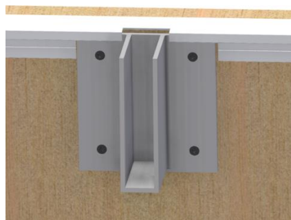
Figure 21 – Glass fin support bracket with upstand top trim
